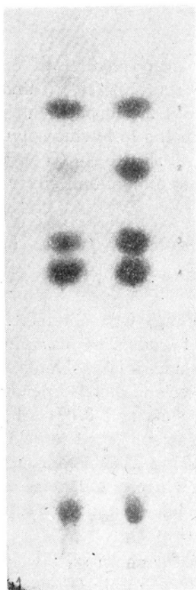
Fig. 1. Paper chromatogram of sugars developed three times with n -butanol—pyridine—water—benzene (5:3:3:1) and detected with ammonium silver nitrate
